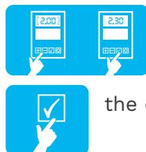
Use the + and – buttons to set the desired tire pressure (max. 5.5 bar) and then press the confirmation button.
